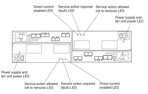
Figure 66. Power supply and fan unit LEDs
